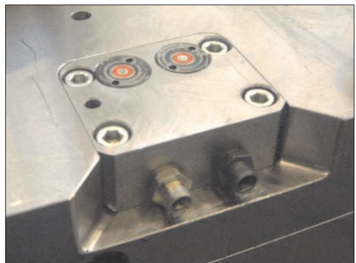
Coupling elements in non-moving tool plate
