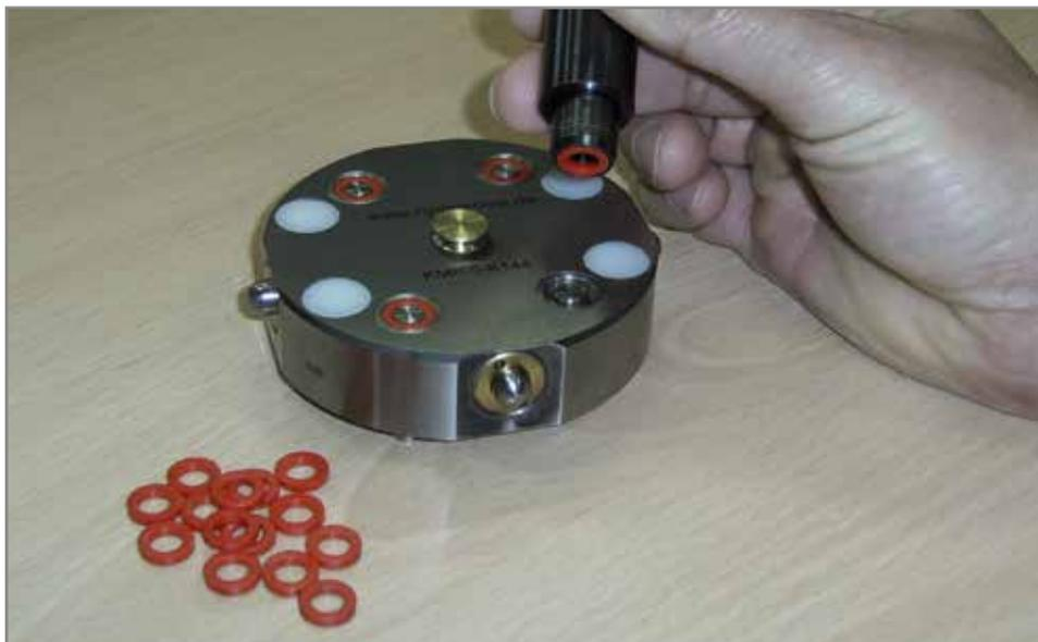
Mounting tool with inserted system seal prior to pressing into the coupling mechanism.
