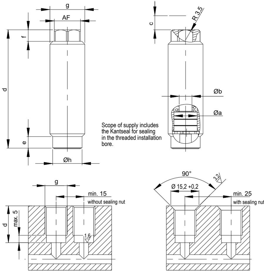
Scope of supply includes the Kantseal for sealing in the threaded installation bore.
