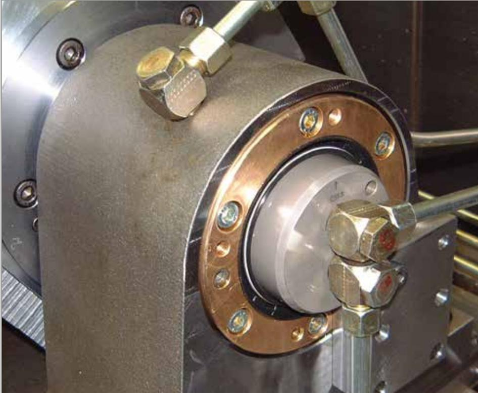
**Application example:** Rotary valve coupling built into the support bearing of a reversible clamping fixture. The design of the rotary valve coupling only permits loading and unloading when the device is turned to a predefined position. This means that it is impossible for the item to become unclamped in the machining positions. Installation in the thrust bearing is extremely compact, saving valuable machining space for the clamping of workpieces.
